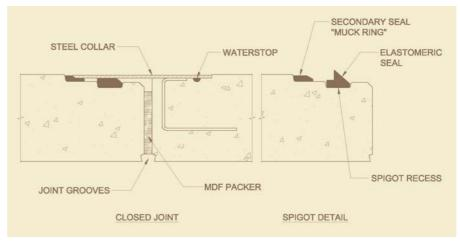
Figure 1. J Series Jacking Pipe Joint.
